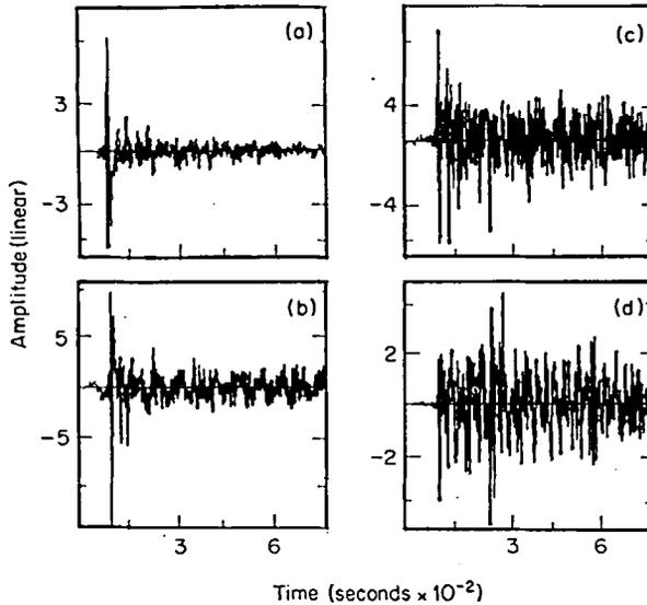
Figure 2. Impulse response functions, recorded in room R2 for increasing source receiver distance: (a) s/r distance = 1 m; (b) s/r distance = 1.5 m; (c) s/r distance = 4 m; (d) s/r distance = 9 m (initial response part is shown).
