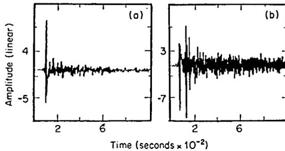
Figure 4. Impulse response functions, recorded in room R2 for varying source/receiver orientation: (a) s/r orientation = 0°; (b) s/r orientation = 90° (initial response part is shown).
