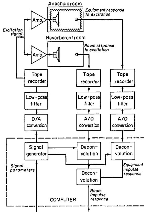
Figure 1. Schematic representation of room response measurement technique.
