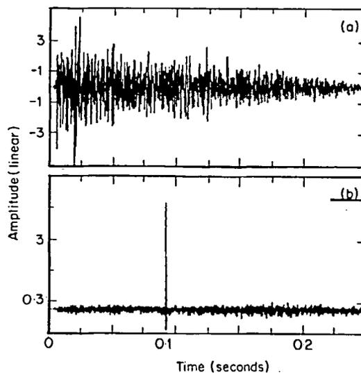
Figure 6. Inversion results for a room impulse response: (a) original response recorded in room R2, for  $s/r$  distance = 9 m; (b) result of inverse filtering applied on this function.
