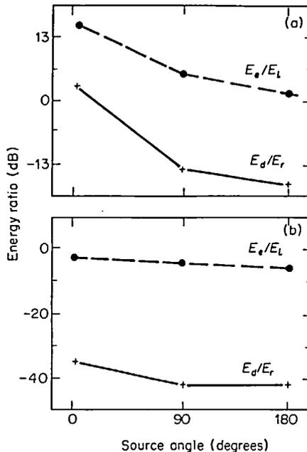
Figure 5. Effect of source/receiver orientation on the response energy ratios: (a) s/r distance = 1 m; (b) s/r distance = 9 m. —, Direct to reverberant ratio; - - -, early to late ratio.
