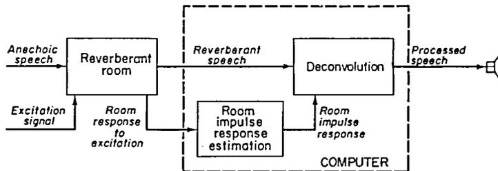
Figure 8. Set-up for the speech processing scheme to evaluate the effect of response inversion.
