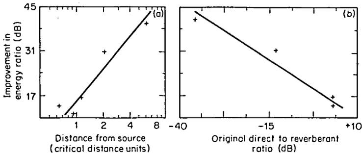
Figure 7. Effect of inverse filtering when the exact impulse response functions are used: (a) energy ratio improvement for the different s/r distance recordings; (b) energy ratio improvements vs. the original energy ratio.
