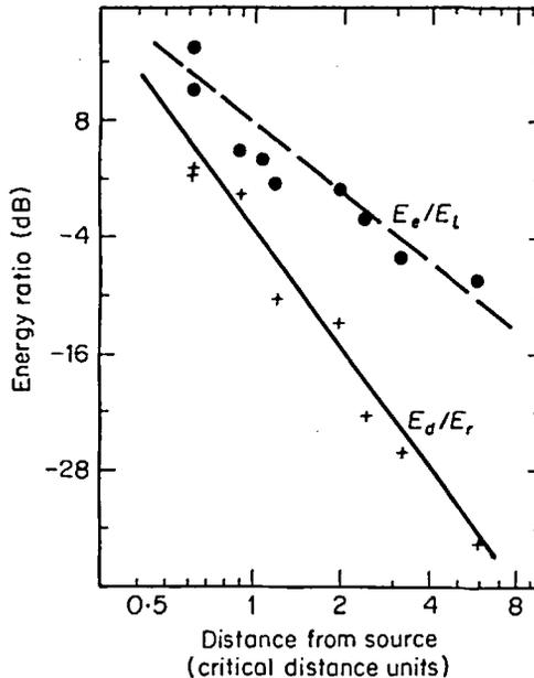
Figure 3. Effect of source/receiver distance on the response energy ratios. —, Direct to reverberant ratio; ---, early to late ratio.
