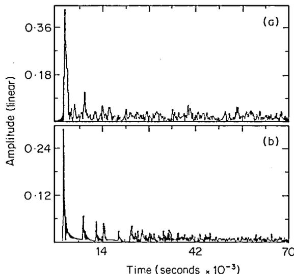
Figure 9. Comparison between the envelope functions for the (a) original recorded response and (b) result of computer simulation, according to the method suggested in reference [11].
